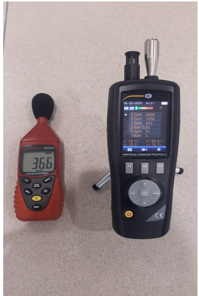
Fig-Measuring Particle Counter & ambient temperature and relative humidity to evaluate air comfort.
