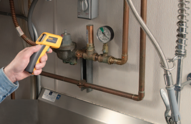
Infrared thermometers are a convenient way to check for temperature differences along pipes that could indicate a moisture leak.
