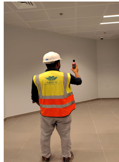
FIG-Using a dBA sound level meter to measure Noise level in indoor room.
